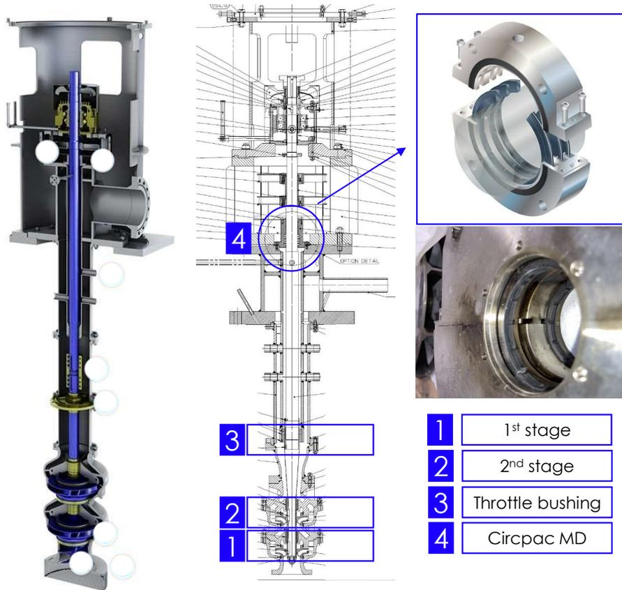
Fig 20. (Left) Sulzer VEY Pump design cross section. (Center) Chloride Validation Sulzer Pump cross section. (Right) Circpac MD Seal.
