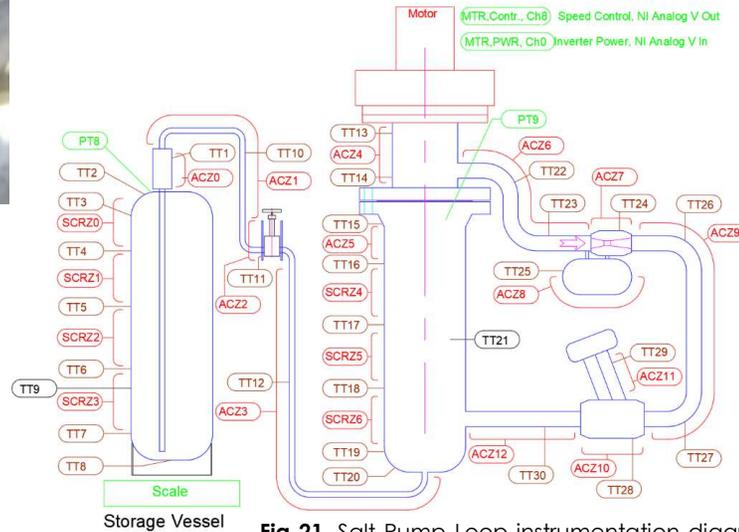
Fig 21. Salt Pump Loop instrumentation diagram with thermal imagery of motor coupling during pump operation at reservoir temperature of 550°C.
