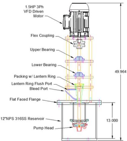
UW small scale lab pump with lantern ring packing seal
