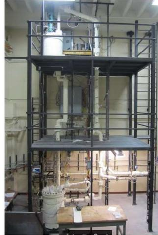
Nagle molten salt pump installed in UW flow loop
