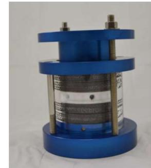
Lantern ring and packing installed in clear stuffing box. (Sepco.com)
