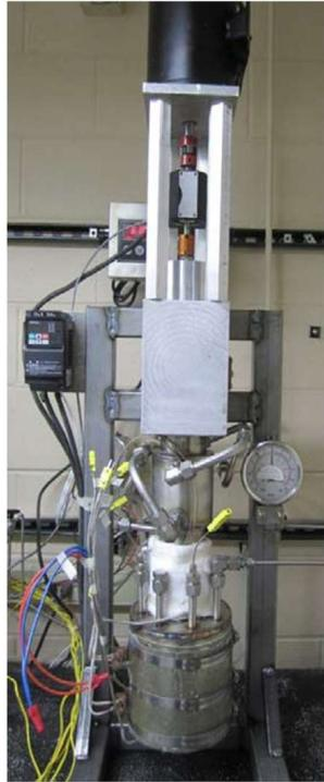
**Fig 12.** (Left) Pin-On-Disk instrumented facilities at UW-Madison & Device detail. (1) Upper assembly components. (2) Components ready for additional welding. (3) Upper bearing housing, shaft, bearing and coupler. (4) Upper bearing housing w/Mag coupler and flex coupler.
