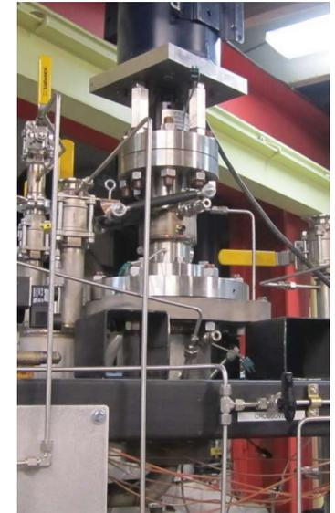
Gen 3 – improved cooling / thermal insulation. Shorter shaft Custom volutes, improved alloys.
