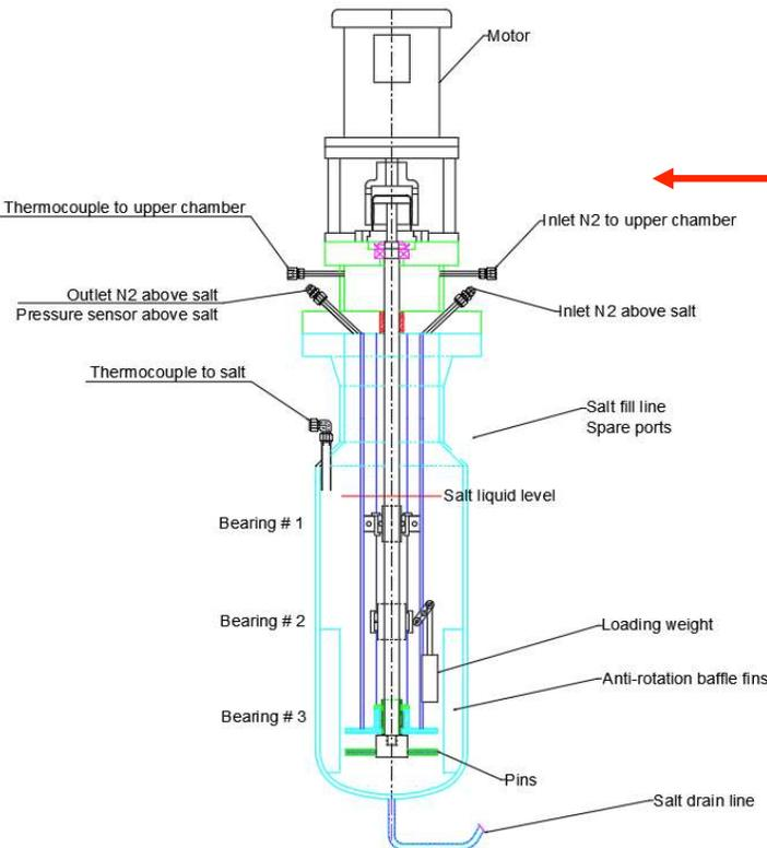
Fig. 16 A. AutoCAD drawing of the Tribology Test Bed structure.
