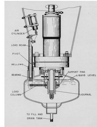
Salt-lubricated hydrodynamic journal bearing tests Nos 1 and 2. (ORNL 58-8-10, 1958, P.G. Smith) INOR 8 – vs- INOR 8
