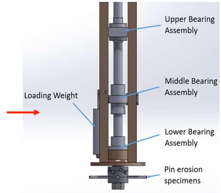
Fig. 16 B. The Tribology Test Bed inner column assembly features three bearing assemblies and a hub for pin specimens
