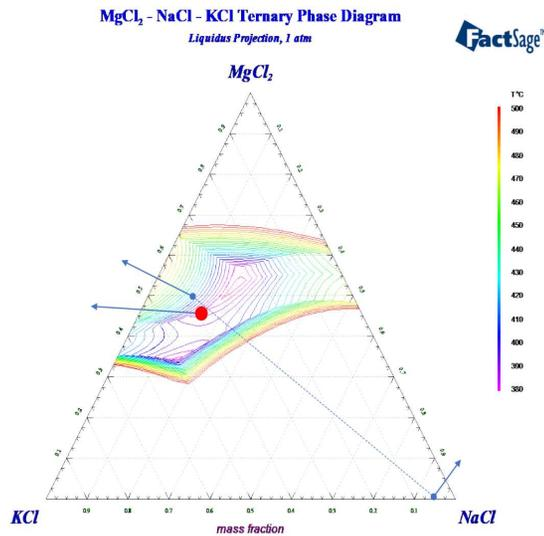
Fig 1. NaCl-KCl-MgCl<sub>2</sub> phase diagram calculated by FactStage showing the composition of the purified baseline salt, AC, and SPK halite. Source [1].
