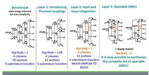
An example flowchart of the steps (layers) followed to create easy-to-operate divided wall columns (DWCs) for fully thermally coupled configurations.
