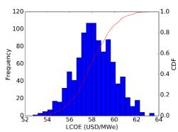
(Left) System design uses liquid sodium in the receiver for excellent heat transfer coupled with molten-chloride salt thermal energy storage. Sensitivity analysis yields a mean LCOE of \$58/MWh
