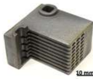
Figure 3. Cross section of the SiC ceramic heat exchanger post densification showing the fluid channels
