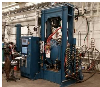
Figure 2. Diffusion bonding furnace installed and operational
