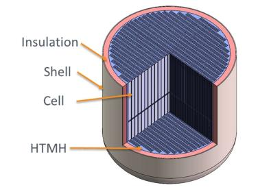
Figure 2. Hypothetical layout of high temperature metal hydride heat exchanger.
