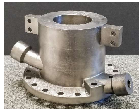
Figure 3 Additively manufactured circulator housing with integral inlet and discharge flow passages
