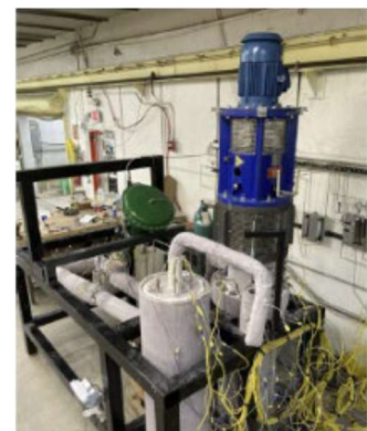
Figure 3 750C chloride salt test loop available for component evaluation at UWisc-Madison
