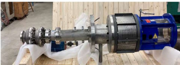
Figure 1. 75 gpm Validation Pump
