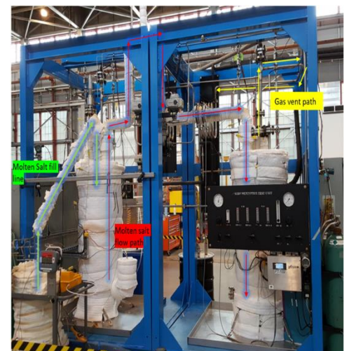
Isothermal Batch Flow Test System
