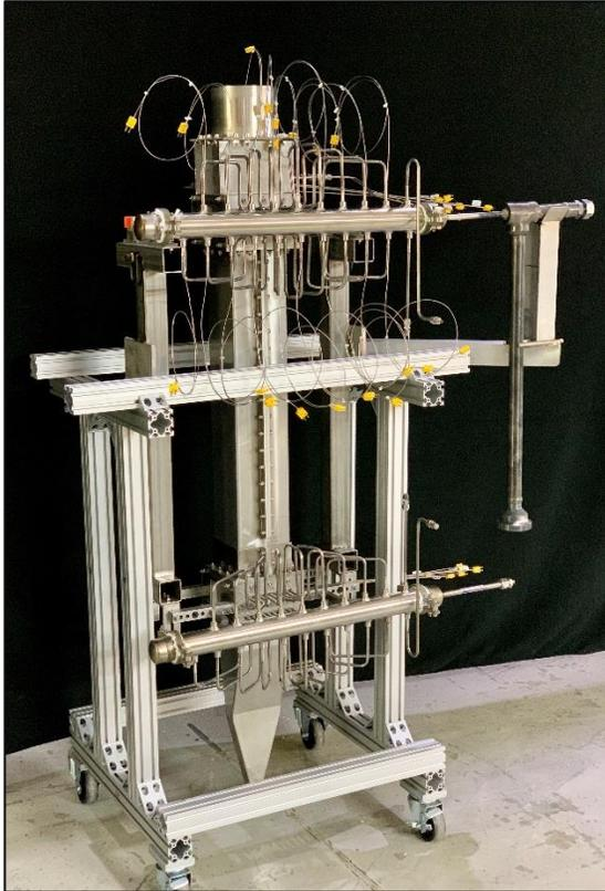
Figure 3 – The 16 kW<sub>t</sub> TES subcore test article.
