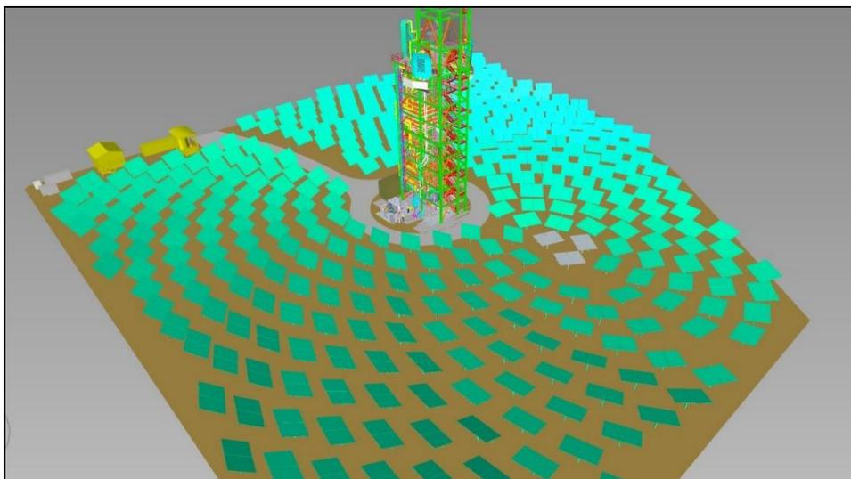
*Figure 1 – The integrated Phase 3 Test Facility, consisting of a central receiver tower surrounded by a field of heliostats.*
