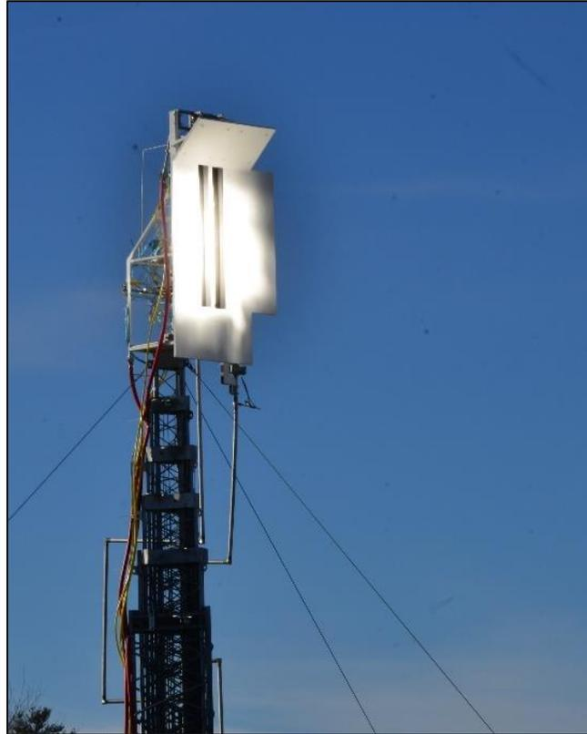
Figure 4 – On-sun testing of the 100 kW<sub>t</sub> receiver test article.
