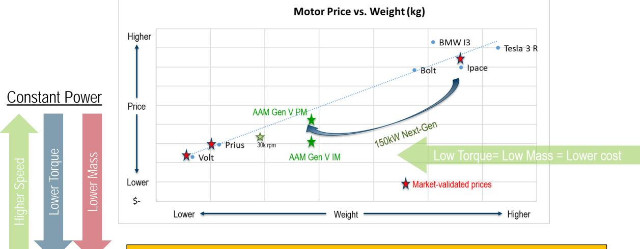
High speed motors can reduce weight and subsequently reduce motor cost
