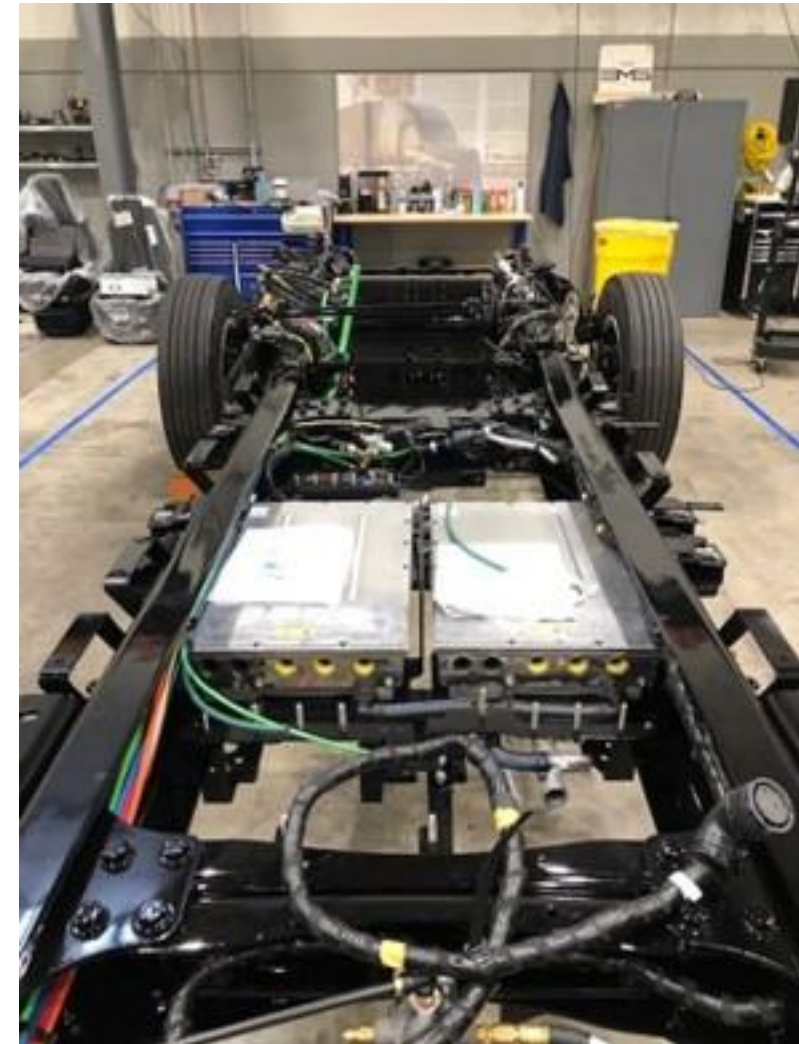
DTNA Freightliner eCascadia glider chassis inverter installation
