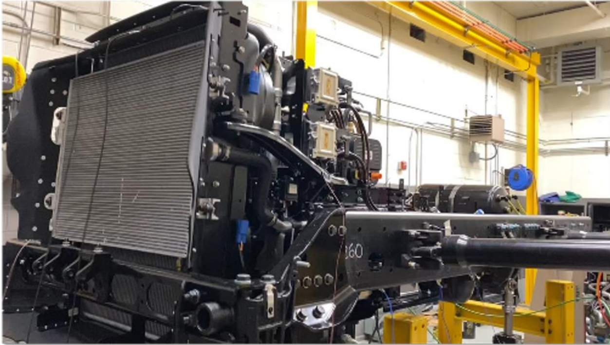
DTNA Freightliner eCascadia 2.0 undergoing component shaker testing
