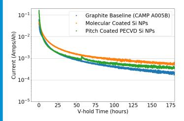
Identified pitch coated electrodes have outstanding calendar life in test cells.
