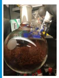
1. Mix Si with petroleum pitch carbon/toluene sol'n (50/50 wt% Si/pitch)
