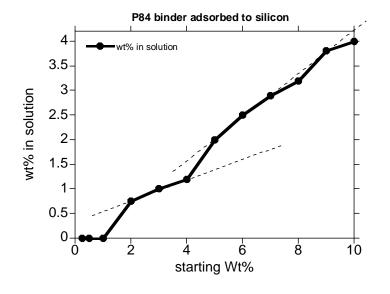
Polymer adsorption isotherms reveal regions of distinct polymer layering – provides guidance to rapidly optimize slurry processing
