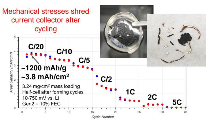
Team is focusing on developing new electrode slurry protocols to facilitate ion transport and mechanical properties.
