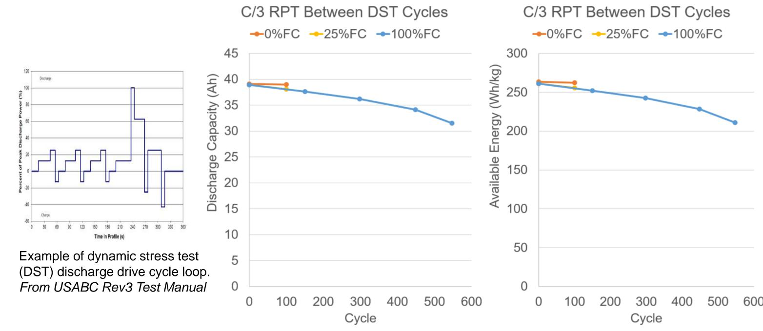
100% fast charge (FC) in under 15-minutes has demonstrated over 500 cycles.
