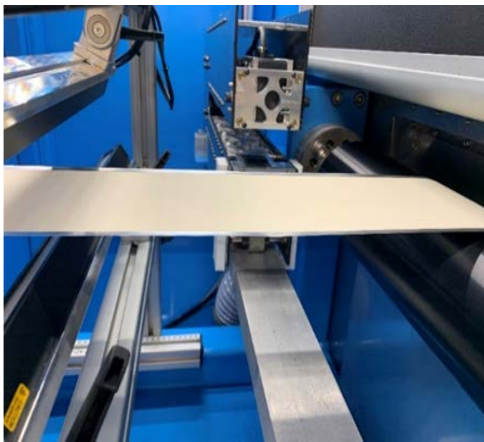
SSE separator coated by a slot-die coater
