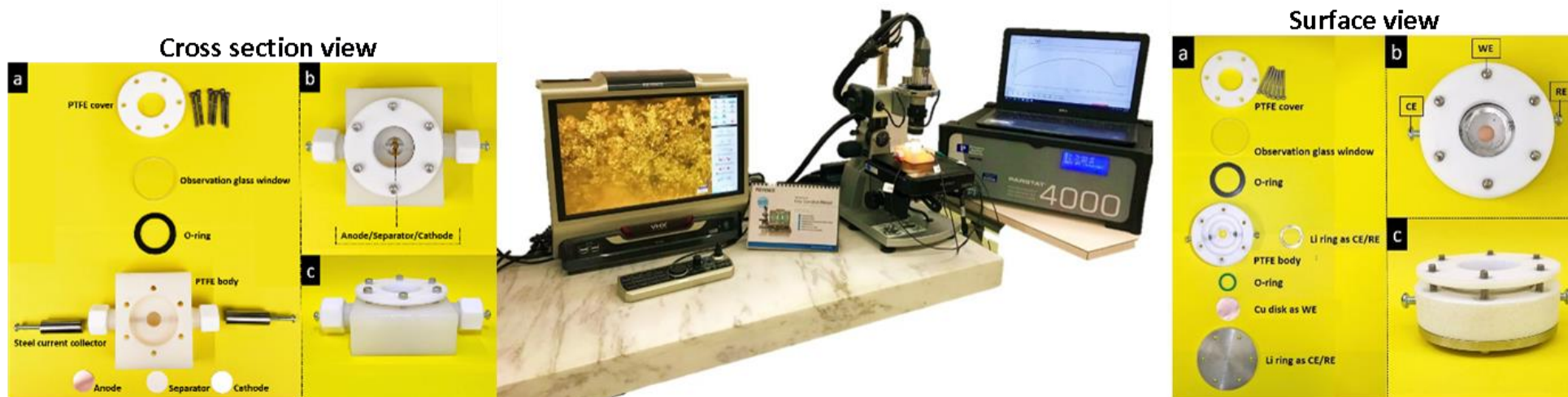
In-situ optical electrochemical cells (left: cross section view; right: surface view) and apparatus (center)
