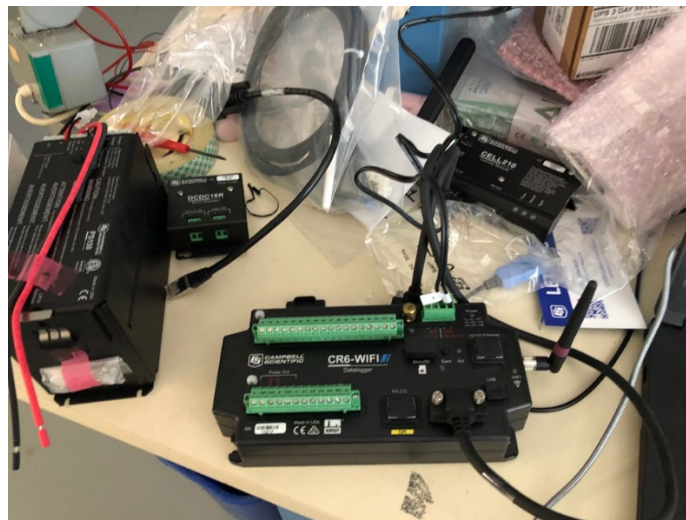
Figure I.22-4. Campbell system components - battery pack, 12-18V boost converter, CR6-WIFI, CELL210 cellular module
