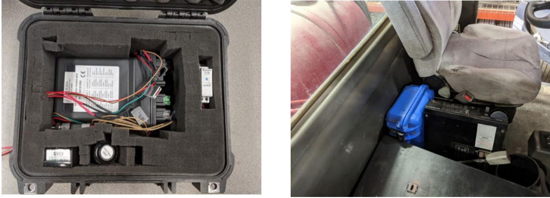
Figure I.22-3. HEM Data Acquisition System components in pelican case and mounted in a truck for testing
