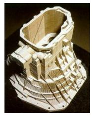
□ This stacking process makes a finished part which is less sophisticated than a SLS or SLM equivalent, but it is cheaper and does not require especially controlled working conditions. Also, if paper is used as the laminate the finished part will be similar to solid wood and can be worked accordingly.
