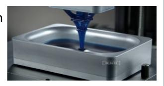
☐ The process is generally faster and a more shallow reservoir of photoresin can be used which also saves on cost. Like with SLA, the finished part has excellent dimensional tolerances and surface finish.
