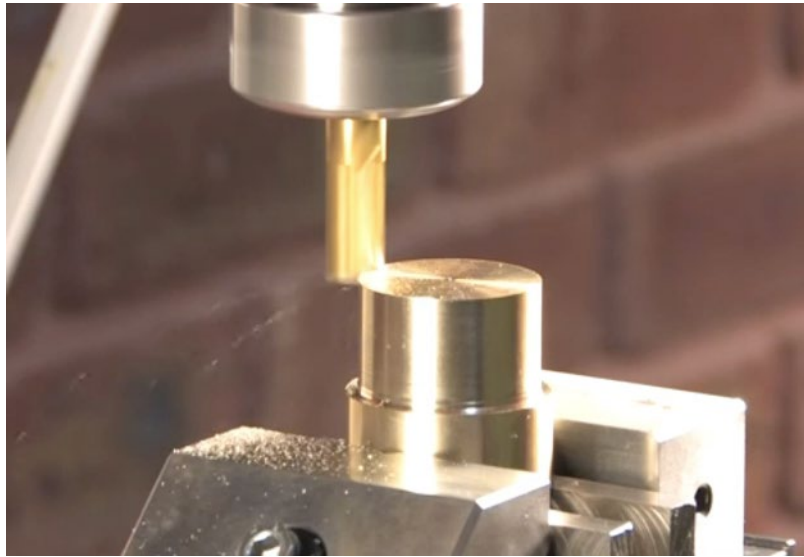
Video: Machining a brass part on a milling machine (mouse-over image to view)
