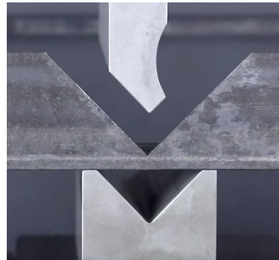
Video: Forming metal stock and sheet metal on hydraulic press (mouse-over image to view)
