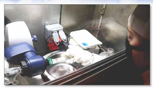
An operations technician removes a tube of thorium-229. Under a newly expanded agreement, EM contractor Isotek will further refine the thorium to provide TerraPower an enhanced purified product to generate Actinium-225 for cancer research and treatment.
