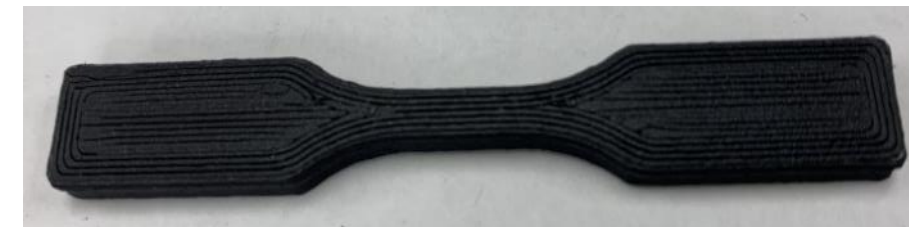
Dog bone printed from 5% wt. CNT-filled Nylon 12
