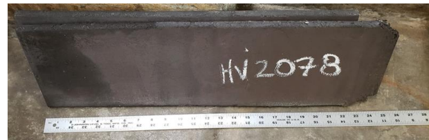
Average grain size = 193 μm
