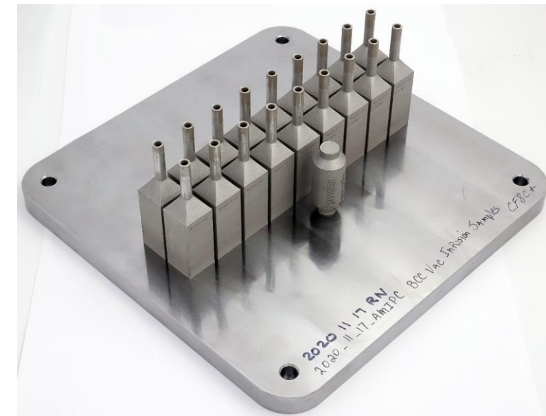
CF8C+ AMIPC preforms with fillet geometry
