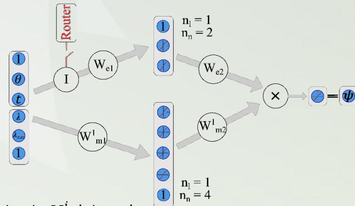
$\psi_j^d(\mathbf{M}_j^i, S_j^i)$  is trained on the basis of a non-kinematic input sets  $\mathbf{M}_j^i$ , internal parameters  $S_j^i$  for the mechanical damage CondNN.  $\mathbf{W}_e$  and  $\mathbf{W}_m^j$  are related to weight matrices of environmental and mechanical damage.
