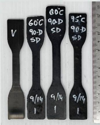
PU specimens after aging in hydrolytic condition after 90 days. Maximum swelling observed in 80C.
