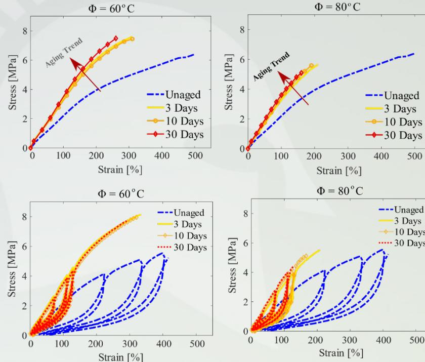
Specimens aged in Dual aging at 60 & 80°C for 30 days for thermo-oxidation at 0%RH for then moved to photo-oxidation for 3, 10, and 30 days.
