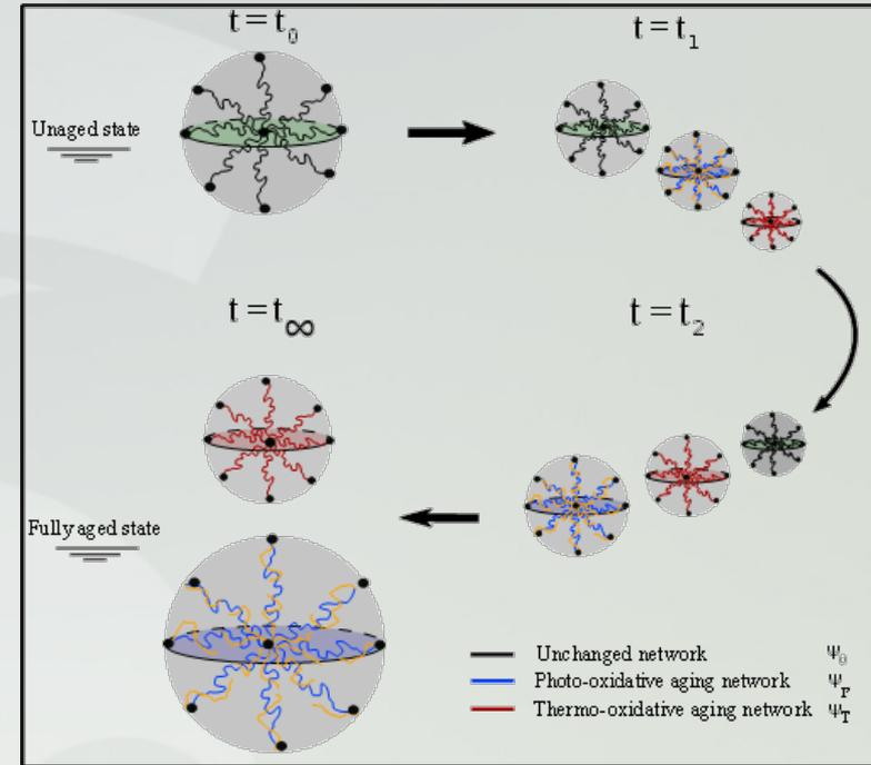
Unaged network ( $t = t_0$ ) continues to change and get replaced by two new-subnetwork at the fully aged state ( $t = t_\infty$ ).
