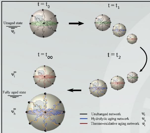
The strain energy of the material in all states of aging,
