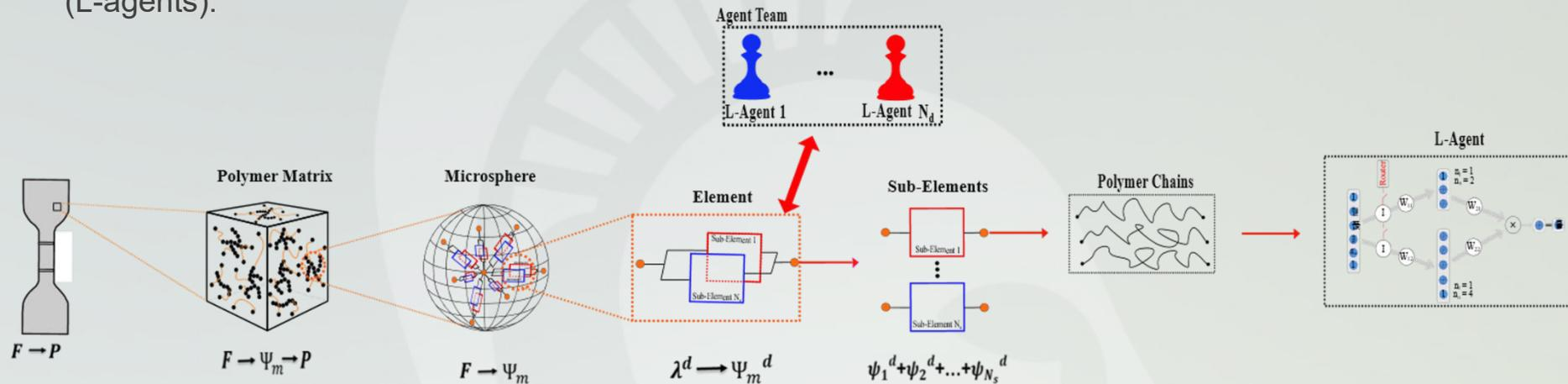
Two – point  $\frac{\text{strain}}{\text{stress}}$  tensors ( $F: P$ )  $\rightarrow E$ : deformation gradients,  $P$ : first Piola – Kirchhoff stress
