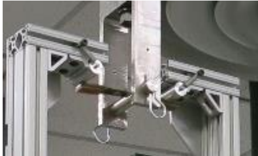
Customized 3-Point Flex Fixture Utilized for Dynamic Testing of Coupons
