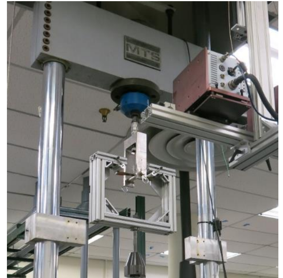
Customized 3-Point Flex Fixture Utilized for Dynamic Testing of Coupons
