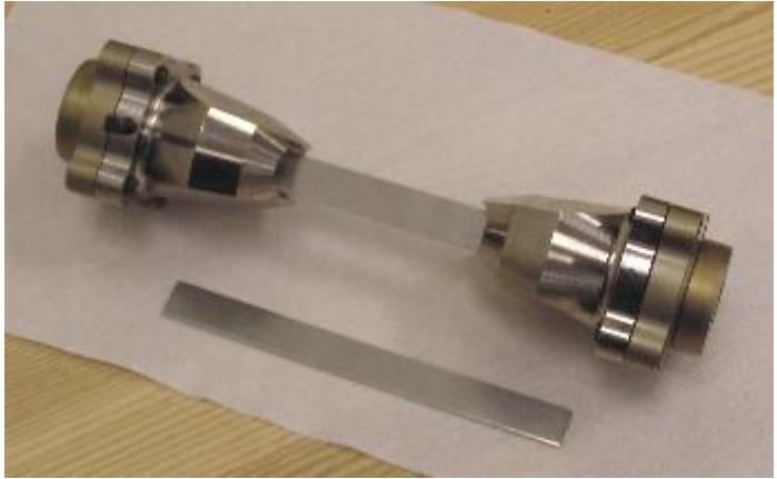
Low-mass grip used in high-rate test machine.
