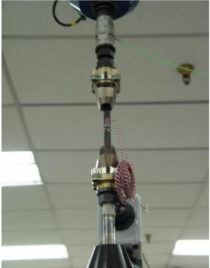
Typical coupon test set-up on high-rate tension machine.
