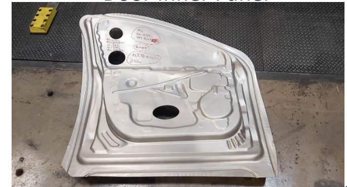
A door outer panel (top) and a door inner panel (lower) fully formed at 250°C using E-Form Plus
