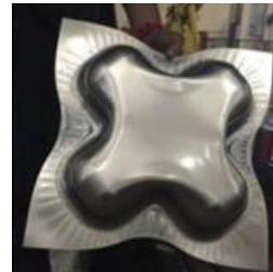
Cross-Form part stamped using E-Form Plus
