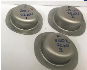
Erichsen cups fully formed using E-Form Plus
