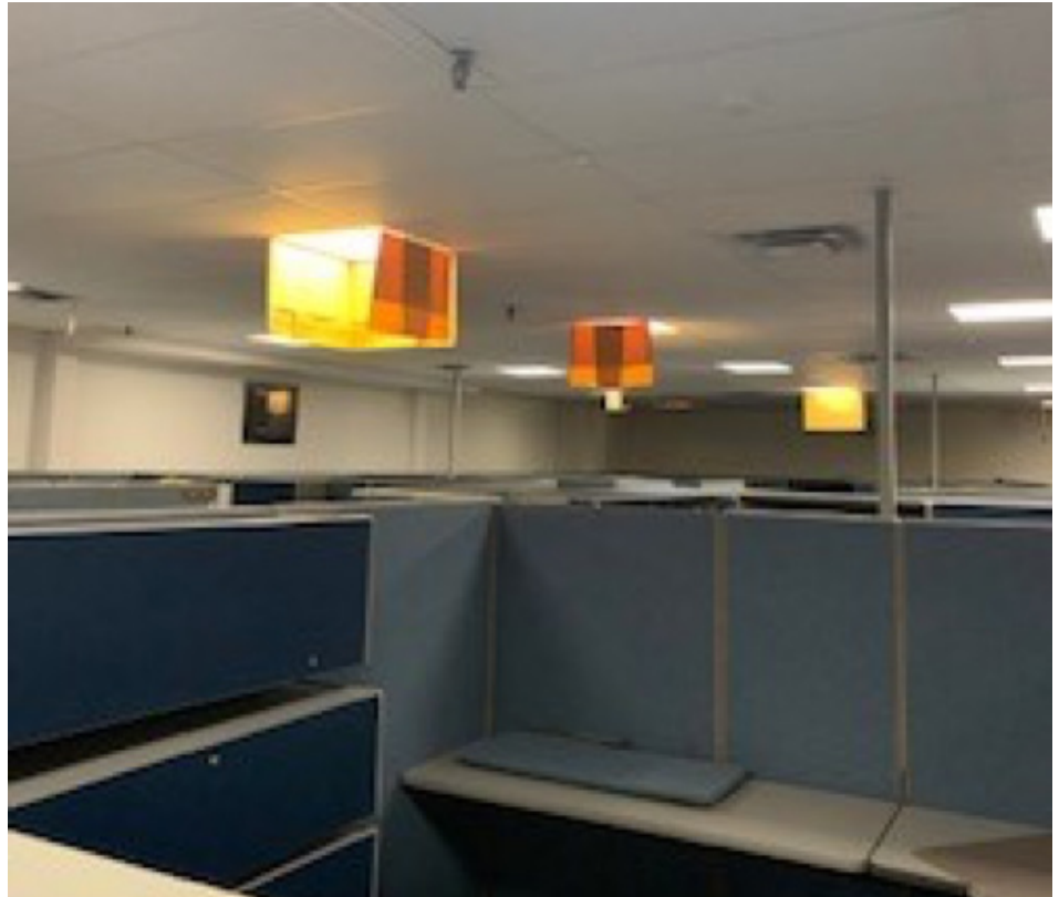
Figure 6. Coping strategy for overhead lighting to reduce horizontal illuminance and/or glare. Image courtesy of PNNL
