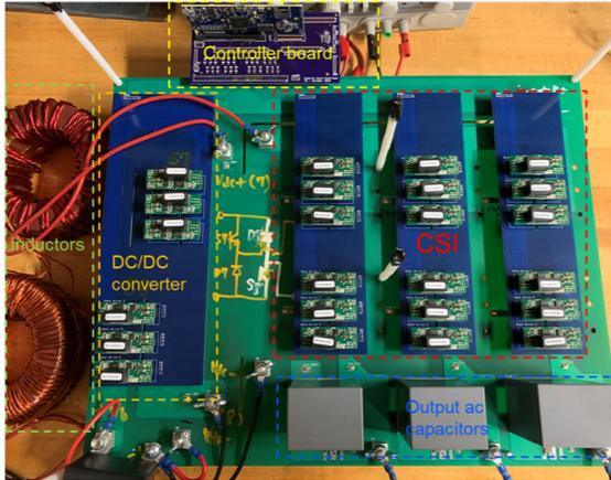
**Benchtop CSI + dc/dc converter testbed PCB**
