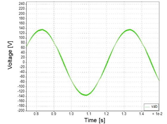
**line-line voltage comparison of CSI benchtop with RL load**
