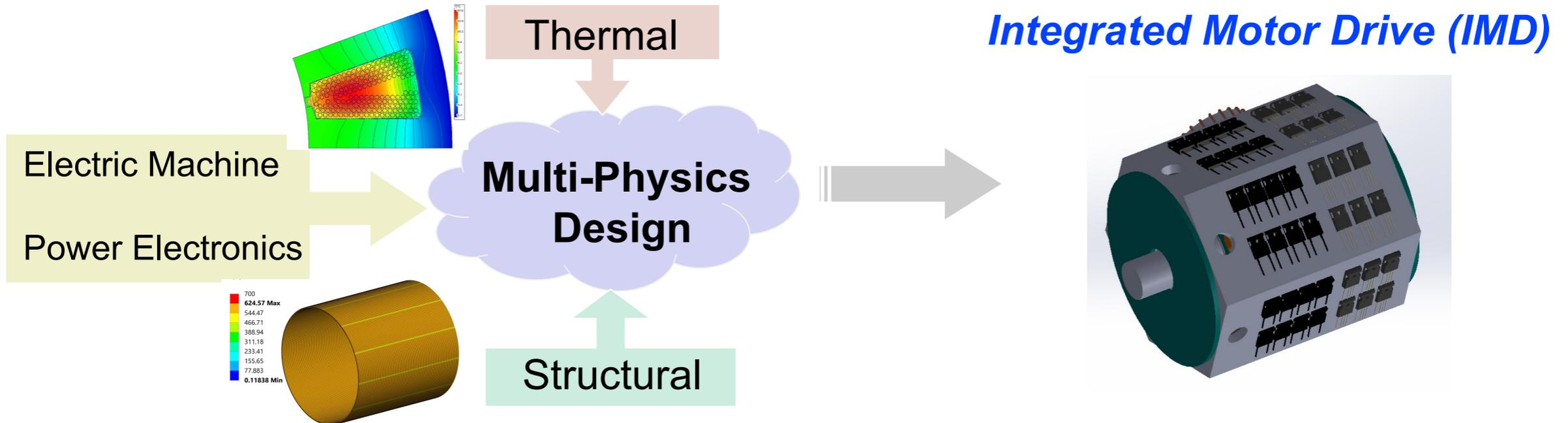
***IMD concept requires aggressive multi-physics design to optimize motor drive system for volumetric power density and cost***
