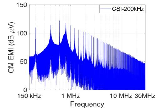
Integral LC filter provides appealing EMI roll-off
