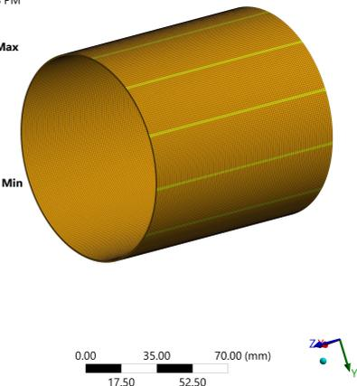
**Critical speed is 75,948 rpm, which is three times higher than the maximum speed of the machine. Maximum stress on the sleeve is 625 MPa, which is smaller than yield stress of sleeve: 2 GPa**
