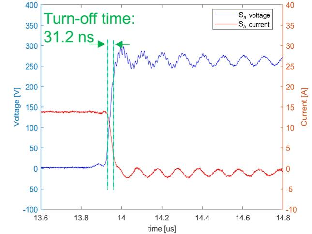
**Current source inverter (CSI)-based double pulse test (DPT)**
