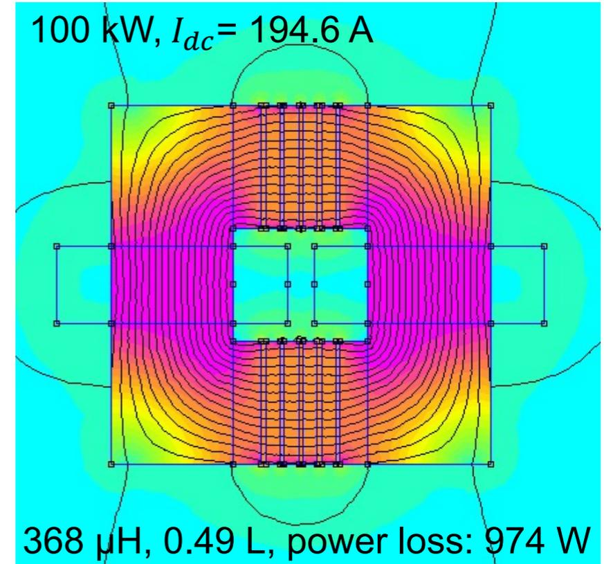
**Minimum volume of 0.49 L is achieved with multi-gapped nanocrystalline core inductor**
