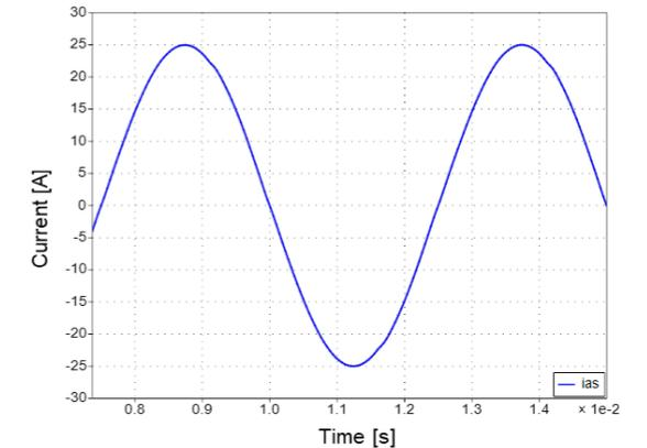
**phase current comparison of CSI benchtop with RL load**
