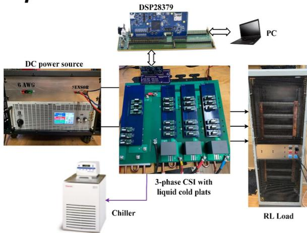
**Block diagram of key testbed components of CSI with liquid cooling**
