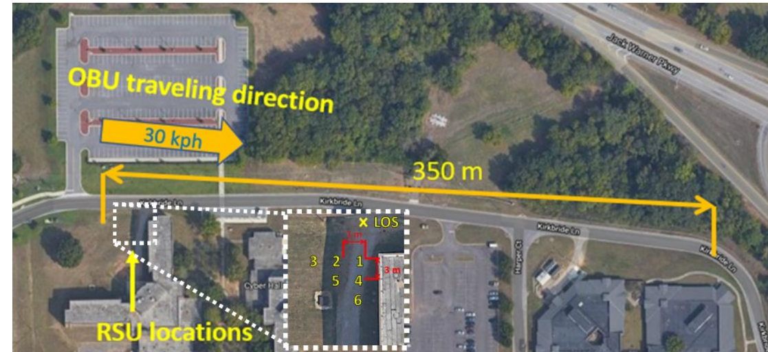
Road test configuration Schematic for RSU locations from LOS to non-LOS positions
