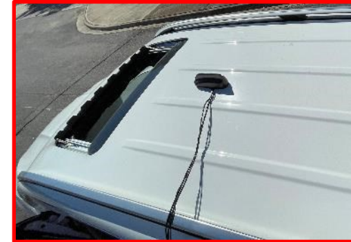
Roof-top antenna for OBU
