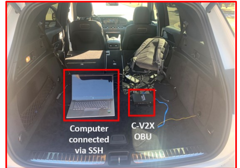
OBU Radio temporarily installed in vehicle
