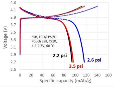
(Disk-in-pouch SSB: 0.1C rate, 2.7-4.2V, 60 °C)
