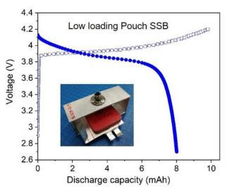
Low loading (1 or 2 mAh/cm²) up to 8 mAh Pouch SSB with LCO cathode has been delivered to DOE for testing.
