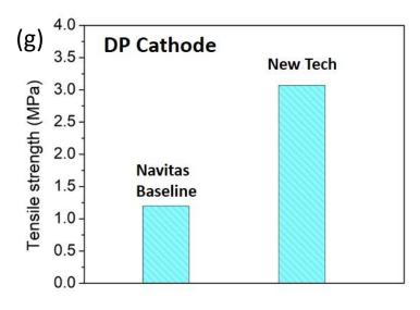
(NMC/Conductive carbon/Carbon additive/PTFE)
