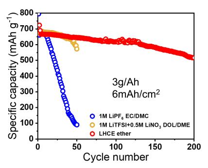
LHCE is the only electrolyte providing sustained cycling stability
