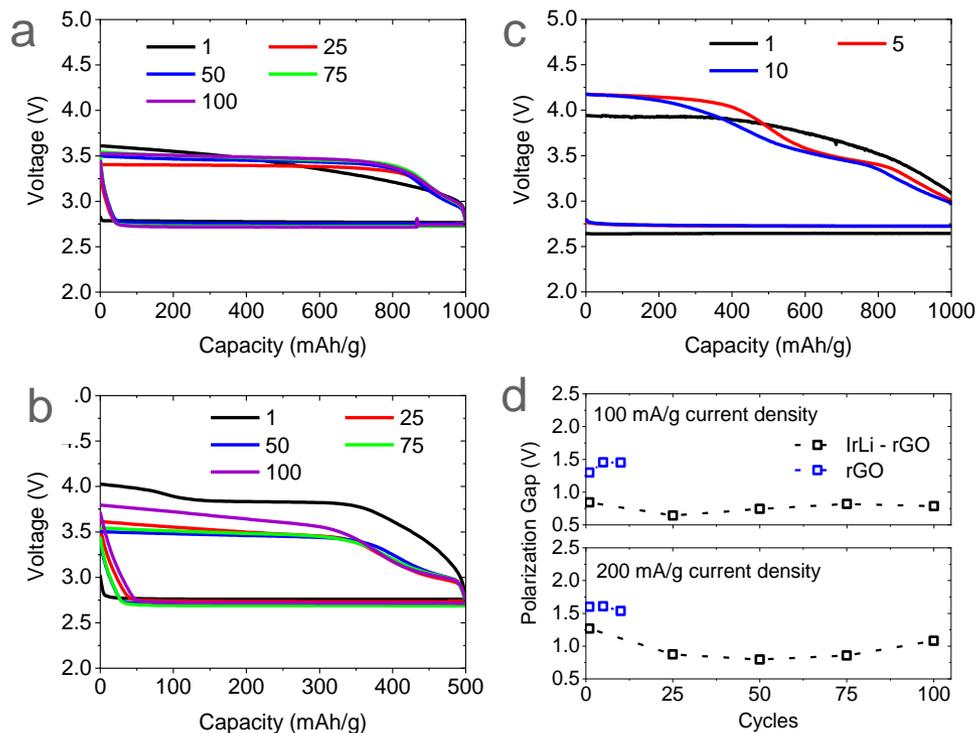
(a) galvanostatic cycling of IrLi-rGO cathode in Li-O<sub>2</sub> cell at a current density of 100 mA/g and a capacity of 1000 mAh/g
