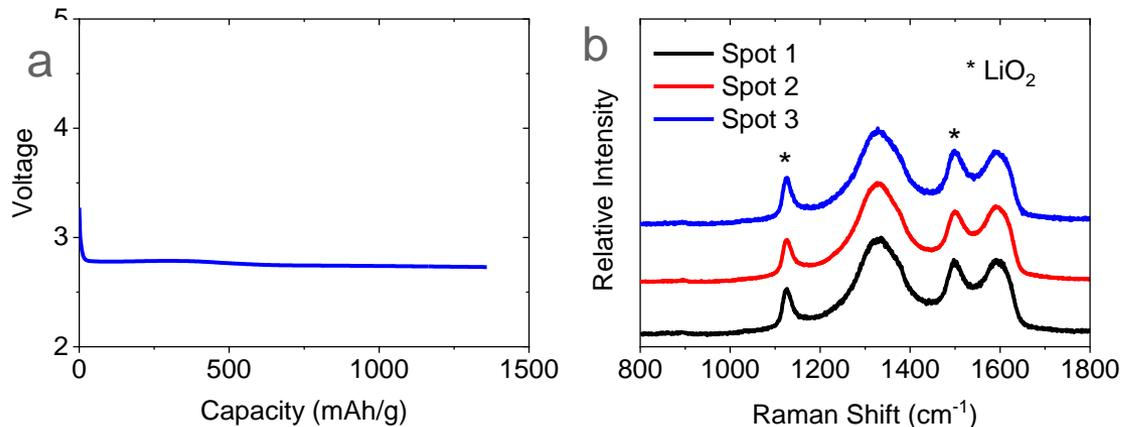
(a) Deep discharge of  $\text{Ir}_3\text{Li}$ -rGO cathode in a  $\text{Li-O}_2$  cell showing the discharge potential  $\sim 2.75$  V for use in characterization
