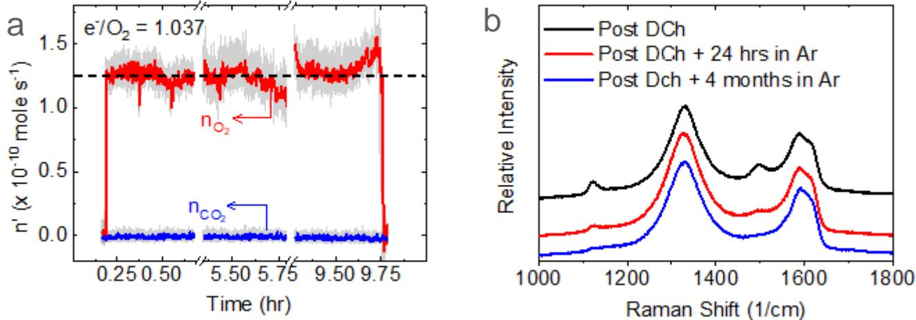
(a) molar quantiles of the evolved O<sub>2</sub> at the 10th charge cycle in three-time intervals (first 30 minutes, mid 30 minutes, and last 30 minutes) calculated from In-situ DEMS experiment of IrLi-rGO cell.
