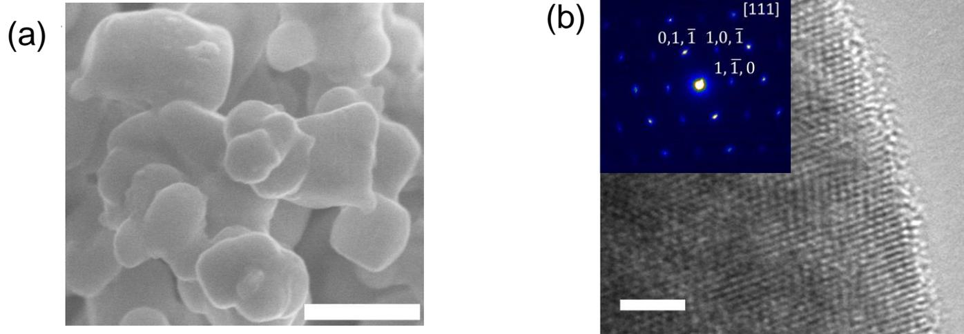
*a) SEM and (b) TEM images of IrLi nanopowder synthesized by thermal treatment of Ir nanopowder and Li foil. TEM inset shows electron diffraction of IrLi particle. Scale bars in a and b are 500 nm and 2 nm, respectively*
