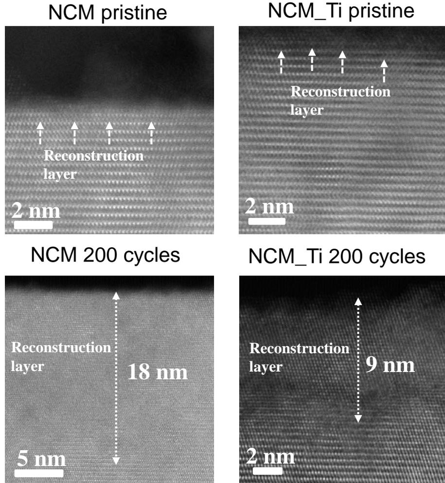
Ti doping leads to the apparent mitigation of the surface reconstruction layer thickness
