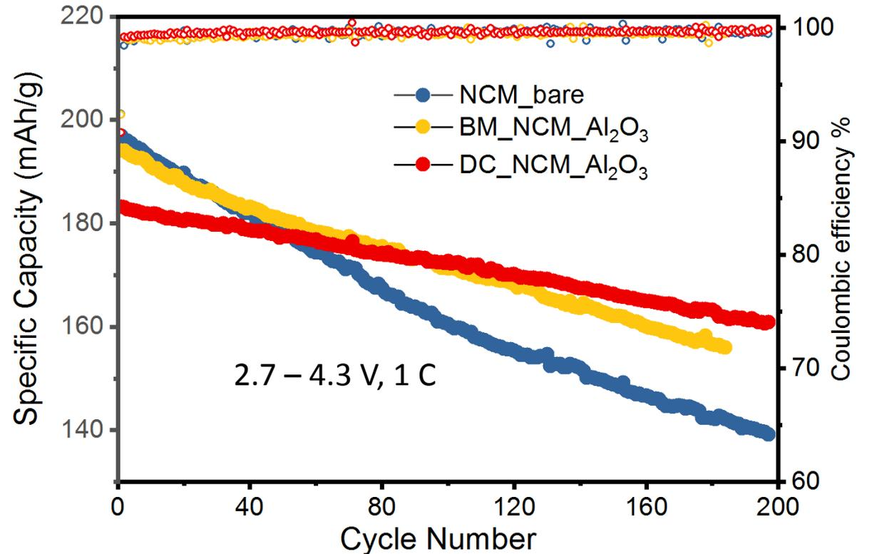
BM\_NCM: ball milling DC\_NCM: dry coating
