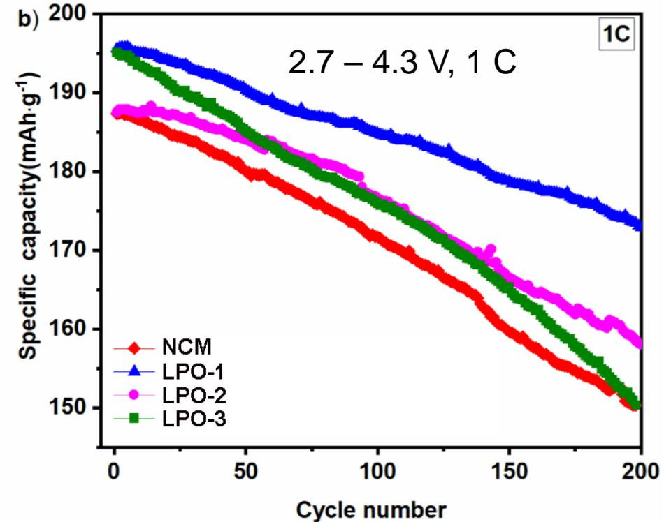
LPO-1 coating shows the highest initial specific discharge capacity and capacity retention.
