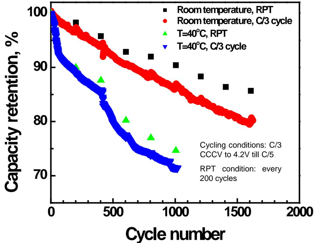
85.7% capacity retentions after 1609 cycles at RT, 74.7% capacity retentions after 1006 cycles at 40°C (RPT condition)
