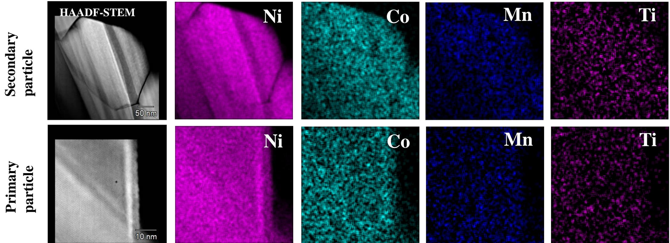
Ti is uniformly distributed at both secondary and primary particle level.
