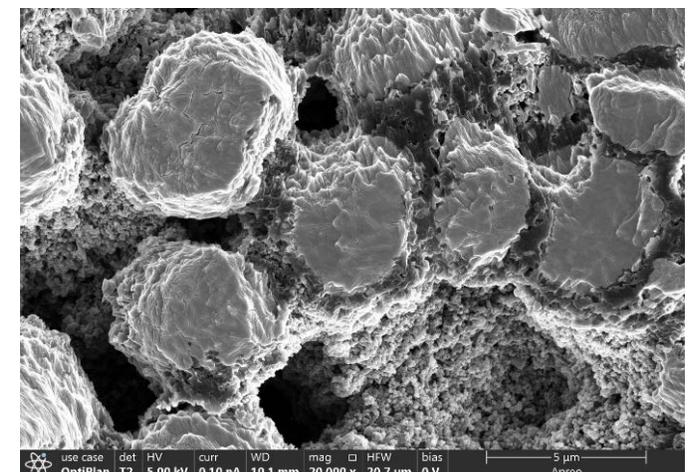
Ti doping can prevent the crack formation and particle destruction.
