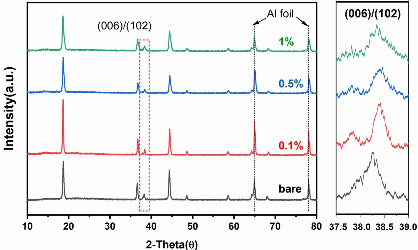
The 0.1% and 0.5% samples exhibit separate peaks (006) and (102) after 200 cycles, indicating a well-preserved layered structure.
