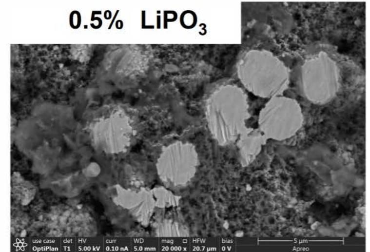
No cracks observed for 0.1% and 0.5% samples after 200 cycles
