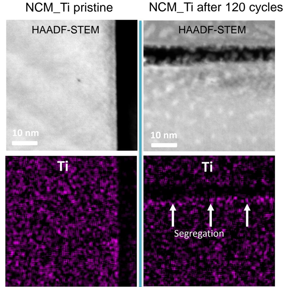
Ti shows uniform distribution in the lattice, and Ti surface segregation can be noticed occasionally
