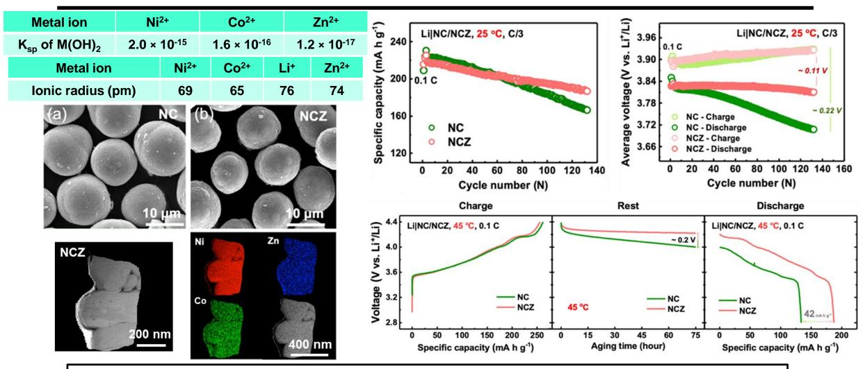
• Zinc can be directly and uniformly incorporated into the coprecipitated hydroxide precursor
