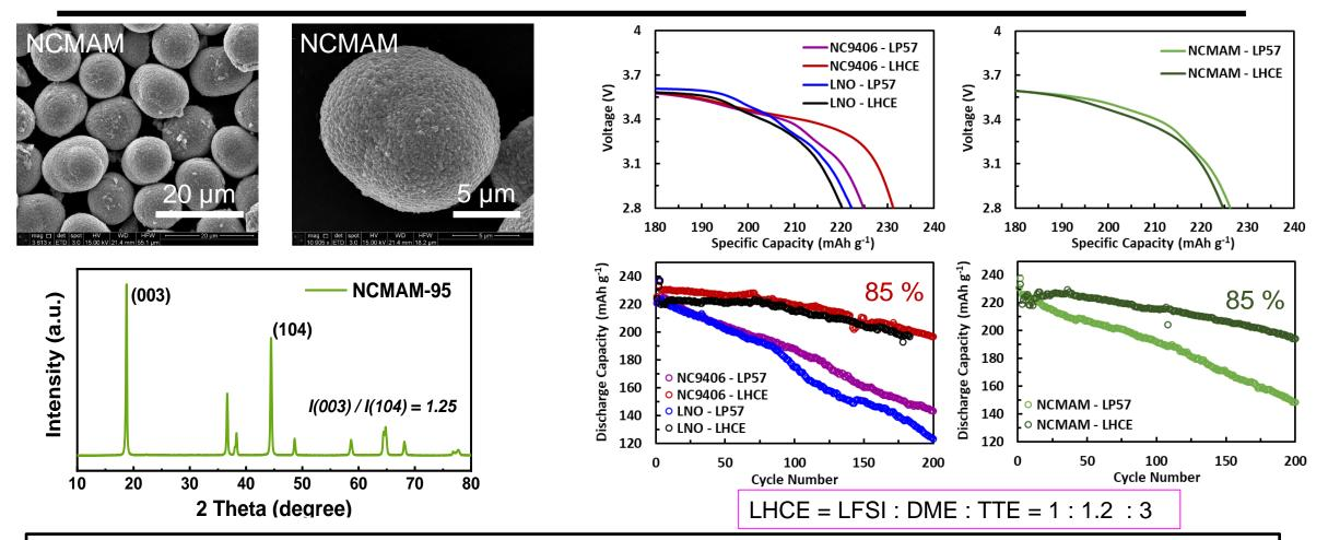
• Several cathodes (e.g.,  $LiNiO_2$  (LNO),  $LiNi_{0.94}Co_{0.06}O_2$  (NC9406),  $LiNi_{0.94}Co_{0.04}Zn_{0.02}O_2$  (NCZ)) and  $LiNi_{0.95}Co_{0.02}Mn_{0.015}AI_{0.01}Mg_{0.005}O_2$  (NCMAM) exhibit high capacities of > 220 mA h g<sup>-1</sup> at C/3
