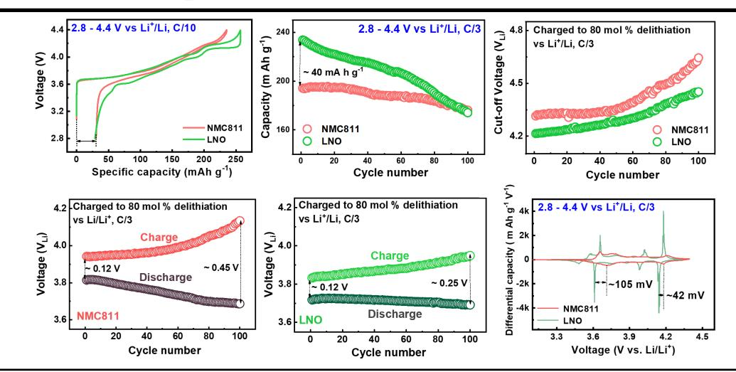
With the same voltage range, NMC811 shows better cyclability than LNO due to a lower degree of Li extraction
