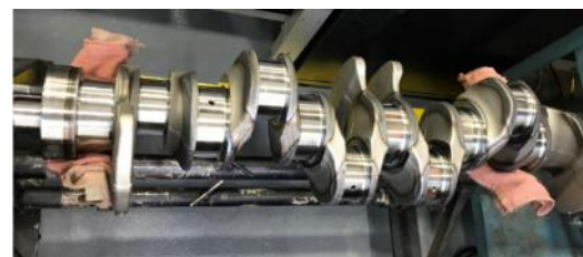
‘Twin-Feed Crankshaft’ for reduced oil flow
