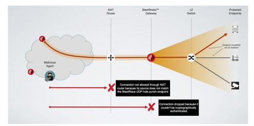
Our solution has been designed with simplicity in mind and deploys as an overlay to the existing network infrastructure. It is also deployed solely as software, either directly on to a server or a user's PC or laptop. In cases where the software instance cannot be installed directly, we can install our software on to any X86 server to act as a secure gateway in front of your critical asset.
