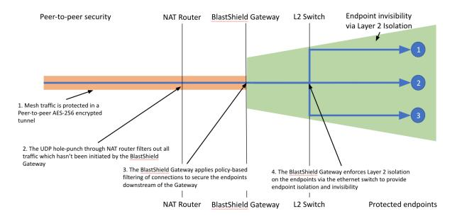
BlastShield<sup>™</sup> endpoints can be any network attached device, thus the following connection pairings can be made:
