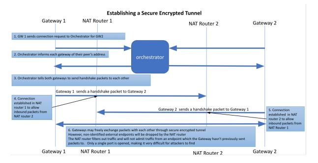
The Orchestrator is only required to set up a tunnel if there are no active sessions currently running or within one hour of the last active session. Unlike traditional SSL VPN's or Cisco's Secure Internet Gateway, the BlastShield<sup>™</sup> mesh solution ensures that there is no single point of convergence that all traffic has to flow through, removing a bottleneck and a single point of failure.
