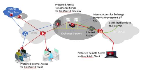
Internal users inside the company's network will access the Exchange Server using their secure encrypted connection, only authorized users by policy will be able to connect.
