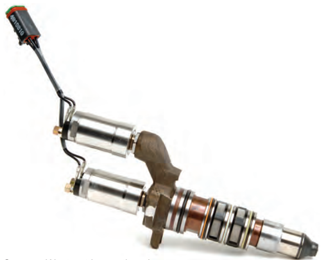
Figure 14-22. High-Pressure Combined Natural Gas and Diesel Fuel Injector
