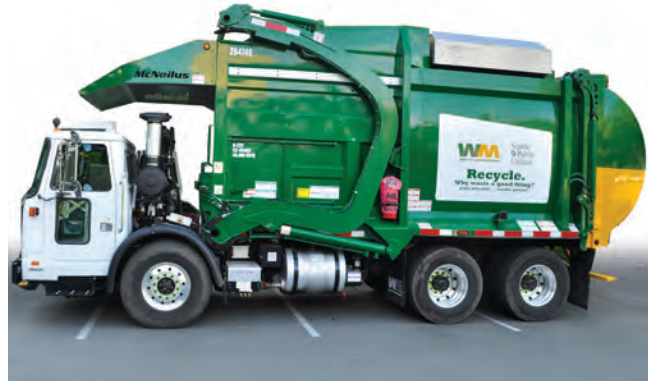
Figure 14-25. CNG Refuse Truck with Roof-Mounted Fuel Storage
