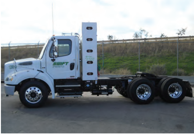
Figure 14-24. CNG Freight Truck with Back-of-Cab Fuel Cylinders
