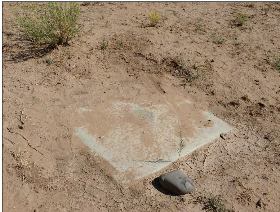
PL-4. Quality Control Monument QC8 Covered with Sediment
