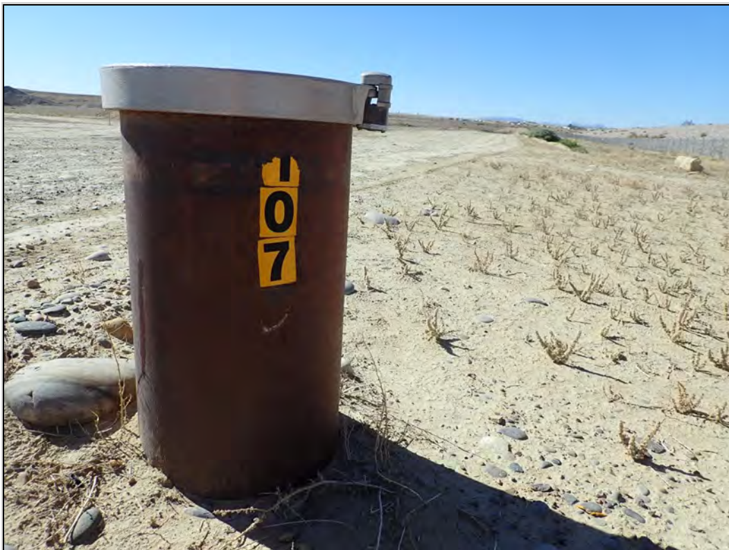
PL-8. Missing ID Stickers on Monitoring Well 1074
