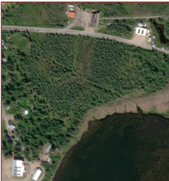
Figure 5: Satellite view image of Northway buildings that have solar panels installed as a result of this project. The solar panels are darker gray rectangles visible on the roofs of the buildings. The washeteria/clinic building is in the upper center; water/sewer garage is located in upper right; and the community hall and addition is visible in lower left corner of the figure. Photo courtesy of Apple Maps.
