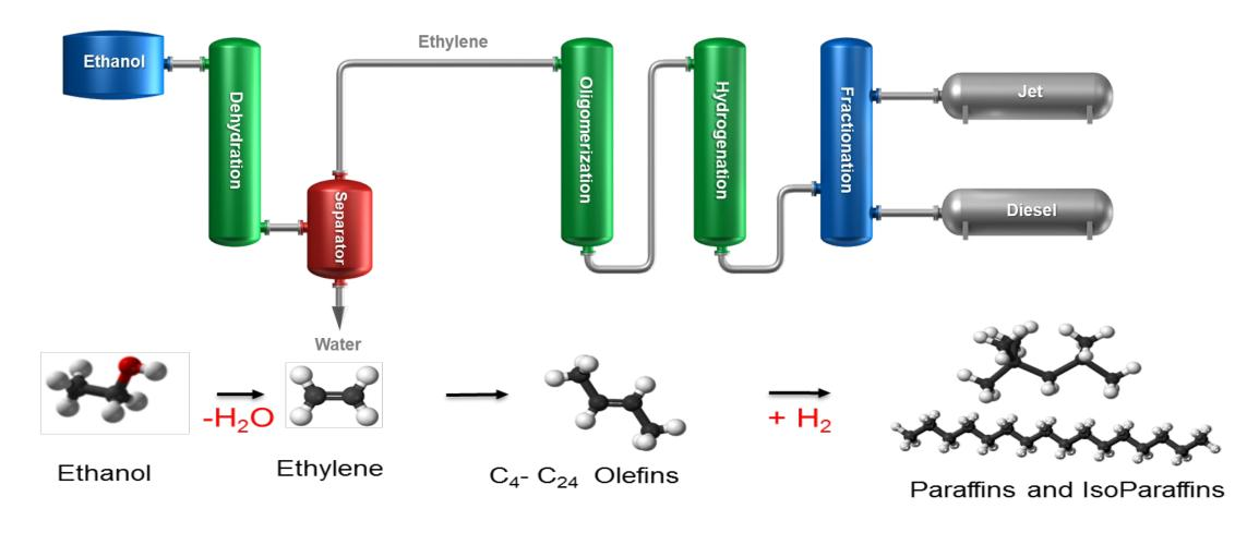
Jet range hydrocarbons ( $C_8$  to  $C_{16}$ ) selectively built
