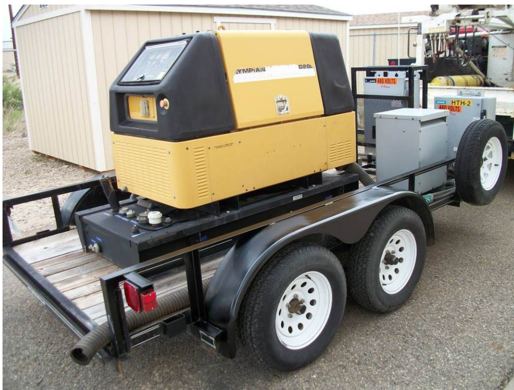
Figure 1. Olympian 20-Kilowatt Generator
