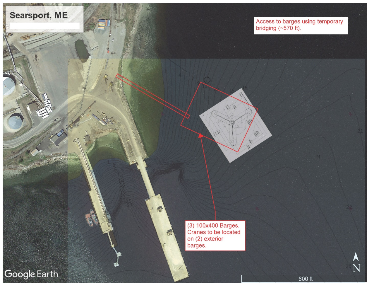
Figure 2.2-21 Assembly of Bottom Segments of Floating Foundation (Configuration of Barges Upon Arrival at Mack Point)
