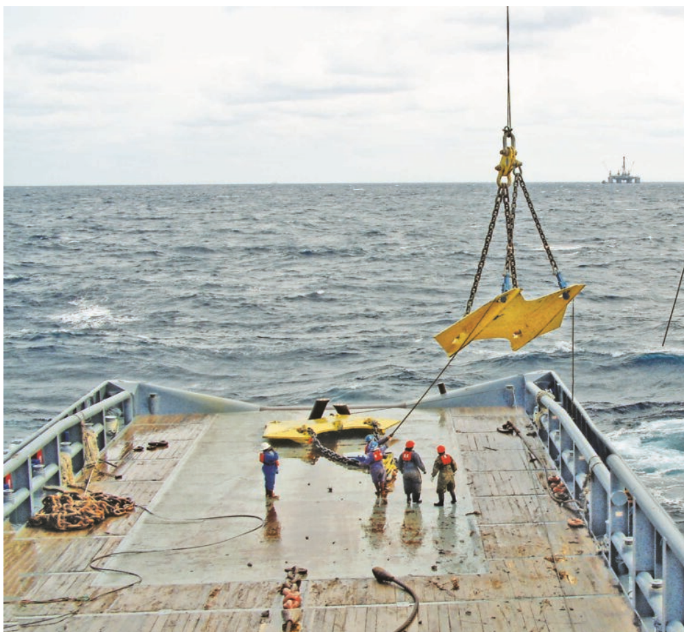
Figure 2.2-10 Example of Vertical Load Anchor
