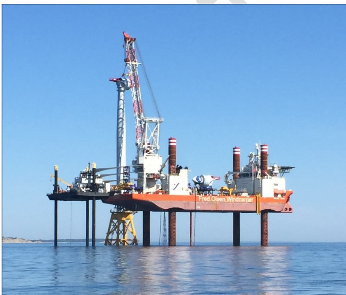
Figure 2.2-26 Example of Turbine Installation Using Heavy Lift Jack-up Vessel (HLV)
