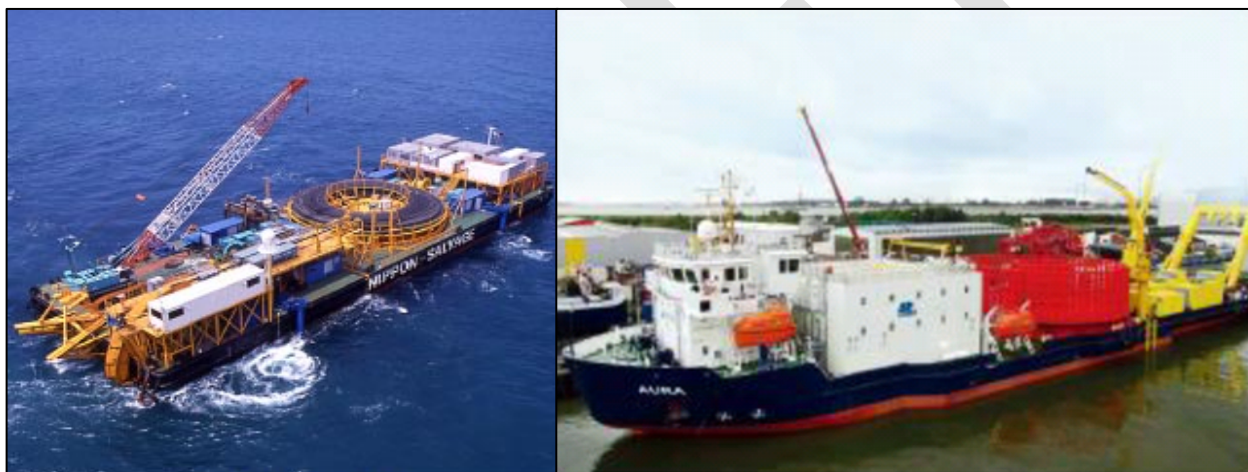
Figure 2.2-27 Example of Cable Laying Barge (Left) and Cable Laying Vessel (Right)
