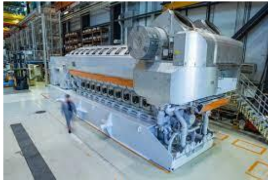
Wartsila 4 stroke engine fueled by NH 3 , 2020
