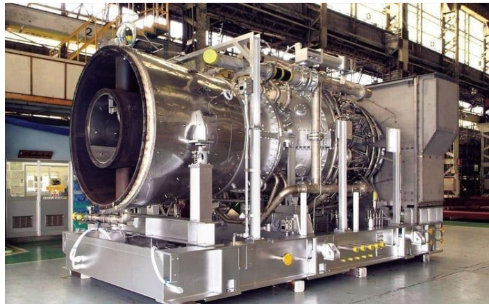
Mitsubishi Power 40-MW class ammonia gas turbine, 2021
