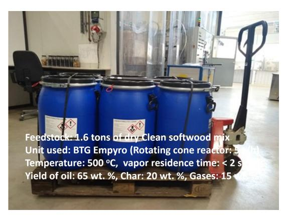
BTG (Netherlands) produced 1 ton (230 gallons of pyrolysis oil.
