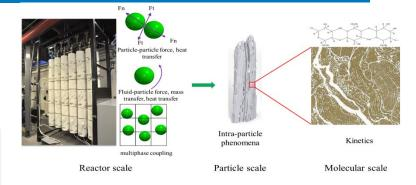
A new approach to kinetic model development: Multiscale modeling + validation across multiple reactors/scales
