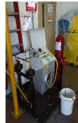
Biogas compression and filling unit (BRC FuelMaker).
