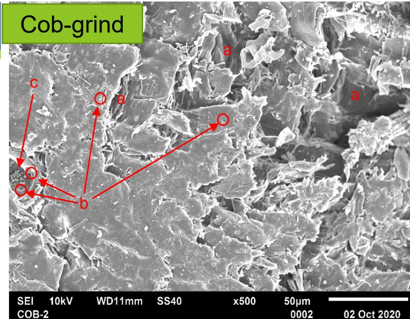
**SEM of cob after grinding**
