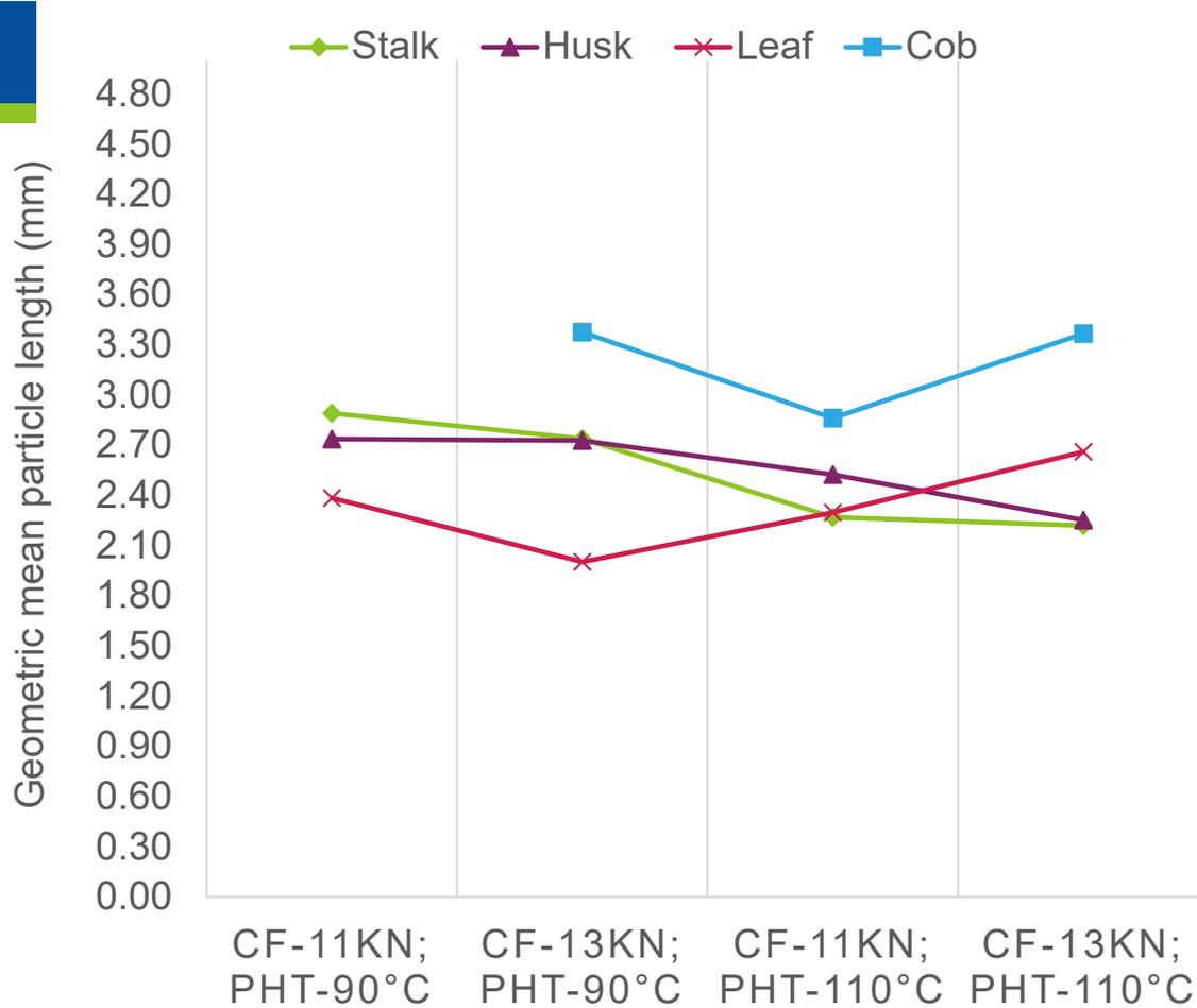
**Geometric mean particle length of particles in corn stover pellets made at different pelleting process conditions**
