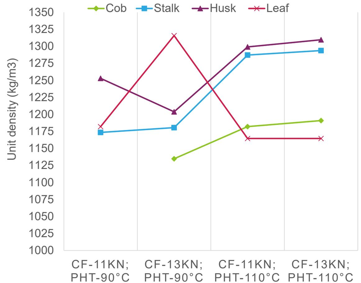
**Unit density of the corn stover fraction pellets made at different pelleting conditions.**
