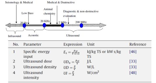
$E_s$ : specific energy in kW s/kg TS (kJ/kg TS); P: power input (kW); T: sonication time (s); V: volume of sludge (L); TS: total solids concentration (kg/L); A: surface area of the probe in cm<sup>2</sup>.
