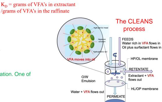
Demonstrated  $K_D$  values of ~ 8 with acetic acid in water during continuous operation. One of the highest ever reported separation efficiencies.
