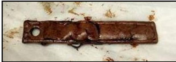
Blistered, delaminated sample after initial 500h test
