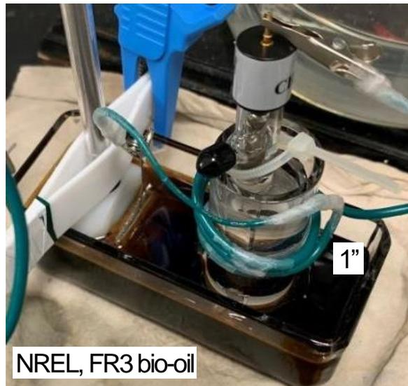
**ORNL custom-design electrochemical cell for bench-top scale EIS measurement**
