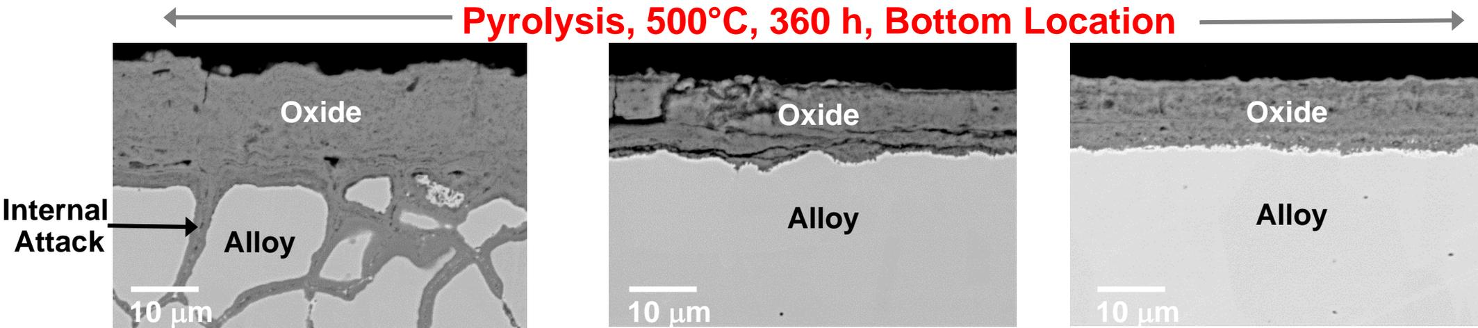
Oxide scales  $\leq 1$  micron thick in air vs  $> 10$  microns thick in pyrolysis reactor
