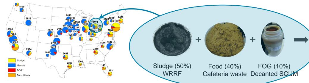
**Objective:** Test regional wet-waste blends to support a 9x increase in HTL plant size while maintaining a 44% yield (2021 milestone). **Progress:** Tested representative, real-world regional blend using
